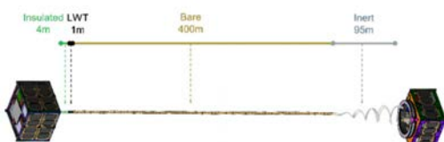
■ Figure 4. Longitudinal structure of the tether
